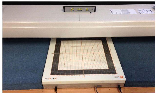
Fig. 1, Set-up showing base-station antenna hanging 8cm above the very-near-field scanner array.
