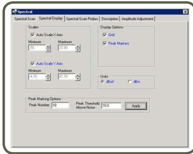
Figure 8 - Spectral Scan Settings for Threshold Value
