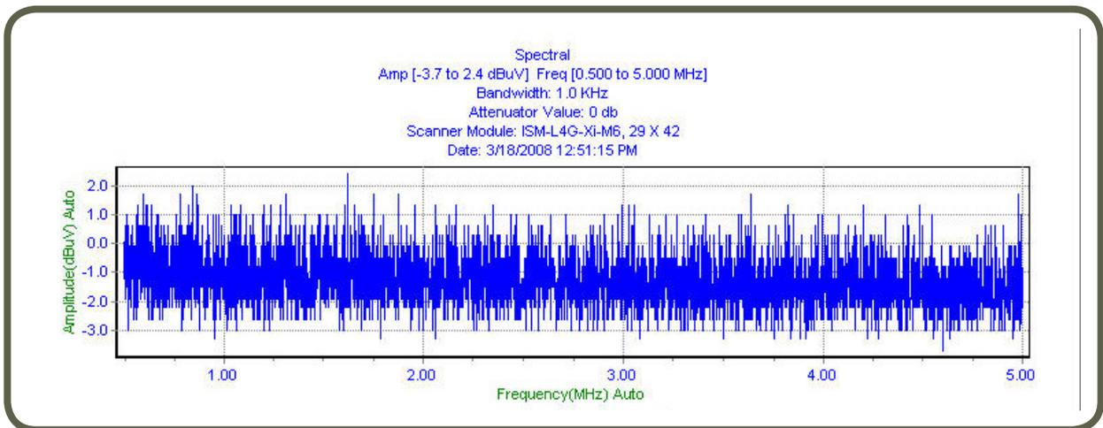
Figure 3 - Uncompensated Spectral Scan with reduced RBW
