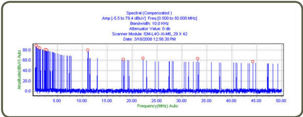
Figure 6 - Compensated Spectral Scan with Source Present and Low Threshold
